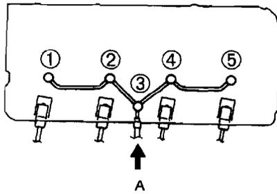
4. Inspect the fuel leak pipe for air leakage.
