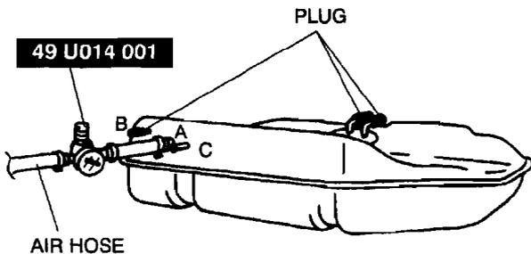
5. Verify that there is airflow from port C when pressure of  $+0.98 \text{ kPa}$   $\{+7.4 \text{ mmHg}, +0.29 \text{ inHg}\}$  is applied to port A.
