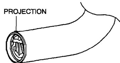
3. If not, remove the nonreturn valve and align the projection with the notch, then reinstall.
