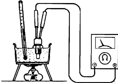
5. Measure the resistance between the engine coolant temperature sensor terminals A and B using an ohmmeter.
