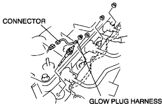
5. Remove the all glow plugs. (Refer to section F2, INTAKE-AIR SYSTEM, GLOW PLUG REMOVAL/INSTALLATION.)
