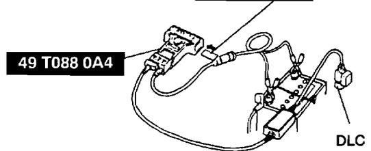
4. Listen to the double beep. The NGS tester is now initialized. Begin the powertrain control system functional test.
