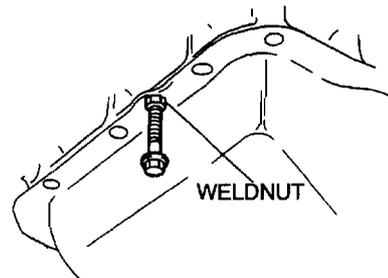
4. Using a separator tool, separate the oil pan.
