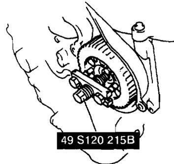
5. Remove the injection pump pulley fixed bolts M8 × 1.25.
