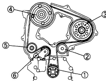
9. Remove the injection pump pulley fixed bolts and camshaft pulley fixed bolt M8 × 1.25.
