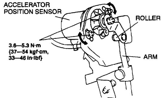
4. If as specified, perform "IDLE SWITCH ADJUSTMENT". If not as specified, perform "ACCELERATOR POSITION SENSOR INSPECTION". (Refer to CONTROL SYSTEM, ACCELERATOR POSITION SENSOR INSPECTION.)
