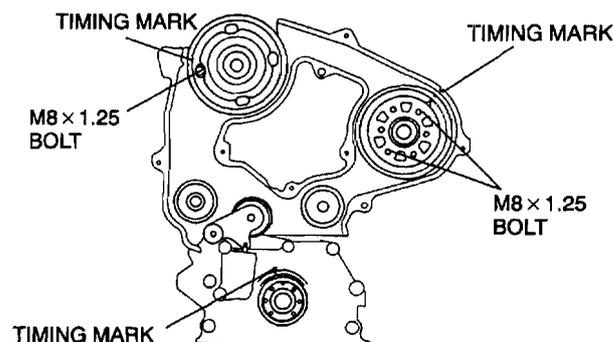
7. If not, align all timing marks according to the procedure below.
