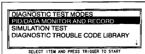
5. Move the cursor to PID values to view. Press the **TRIGGER** key. A star symbol will appear next to the item when it is selected.
