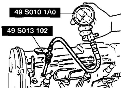
7. Crank the engine and note the maximum gauge reading.
