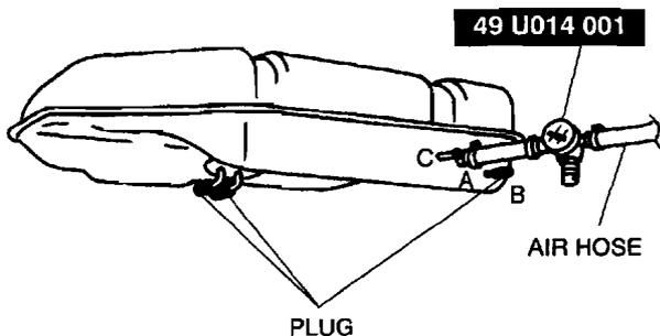
8. Verify that there is no airflow from port C when pressure of  $+0.98 \text{ kPa}$   $\{+7.4 \text{ mmHg}, +0.29 \text{ inHg}\}$  is applied to port A.
