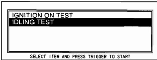
6. The screen will display a list of simulation item. Select the appropriate simulation item for testing, then pass the **TRIGGER** key.
