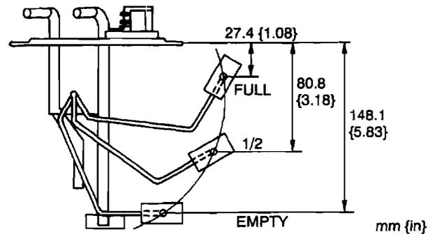
3. If not as specified, replace the fuel gauge sender unit.
