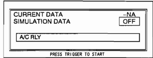
9. The simulation is performed for **3 seconds**, and a **"SIMULATION ACTIVATED PLEASE WAIT"** message is displayed during those 3 seconds.
