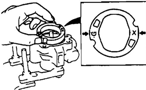
2. Install the vanes in the rotor with the rounded edges outward.
