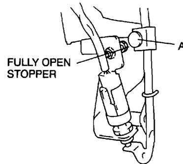
2. Confirm that the voltage of the PCM 2F terminal (accelerator position sensor) is within specification.
