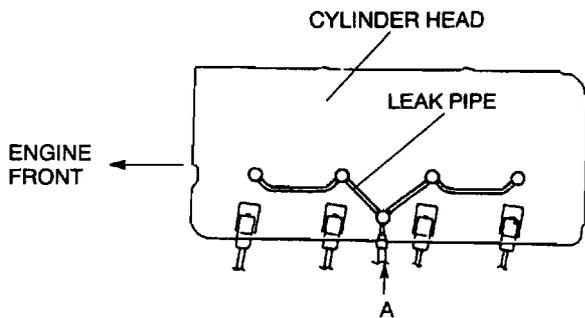
2. Apply soapy water to the joint area of the leak pipe and the injection nozzle, and verify that there is no leakage.
