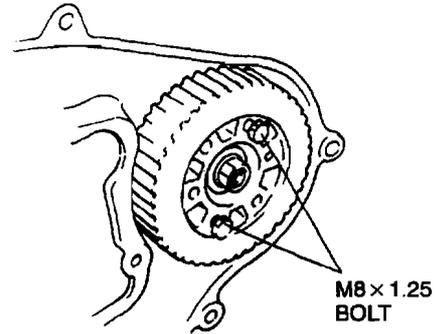
3. Loosen the injection pump pulley lock nut.
