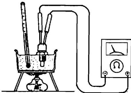
4. Measure the resistance of the IAT sensor using an ohmmeter.
