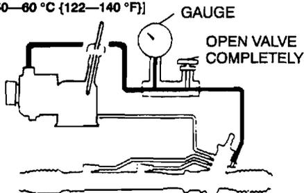
8. Remove the gauge set. Install and tighten the pressure pipe to the specified torque.
