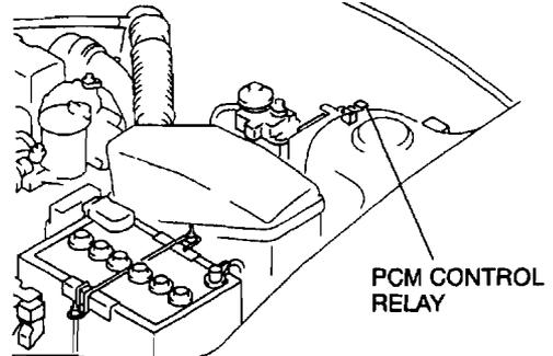
3. Inspect for continuity between terminals of the relay using an ohmmeter.
