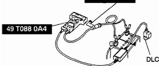
2. Access RPM PID. Press the trigger key to enter this selection. (Refer to ON-BOARD DIAGNOSTIC SYSTEM, PID/DATA MONITOR AND RECORD PROCEDURE.)
