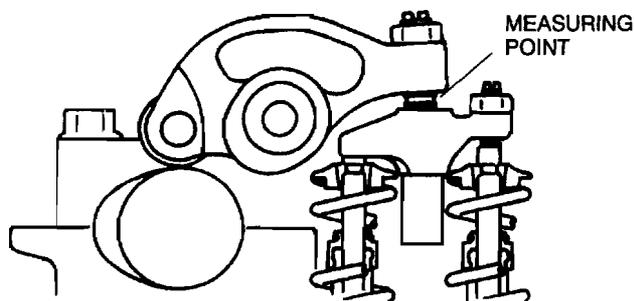
4. If the valve clearance is not within the specification, adjust the valve clearance. (Refer to VALVE CLEARANCE, VALVE CLEARANCE ADJUSTMENT.)
