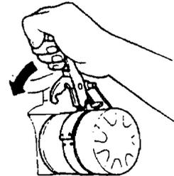
2. Tighten the filter according to the installation direction on the side of it or packing box using the filter wrench.
