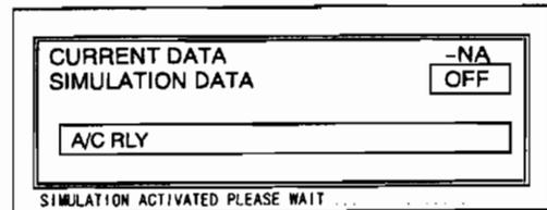
10. To perform the simulation again, press the **TRIGGER** key. To exit the idling test, press the **CANCEL** key.
