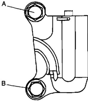
12. Remove the pin from the auto tensioner to apply tension to the belt.
