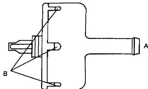
3. Visually inspect that there is no damage nor crack on the evaporative chamber.
