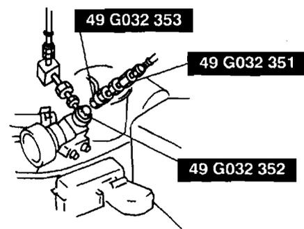
2. Disconnect the pressure pipe from the oil pump, and connect the SST.
