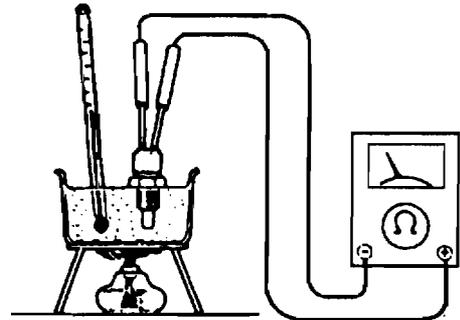
4. Measure the resistance between ECT sensor terminal C and body ground using an ohmmeter.
